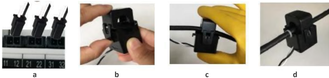
Figure 2-14 5A/2mA, 100A/40mA, 200A/40mA or 400A/40mA SCCT Installation
