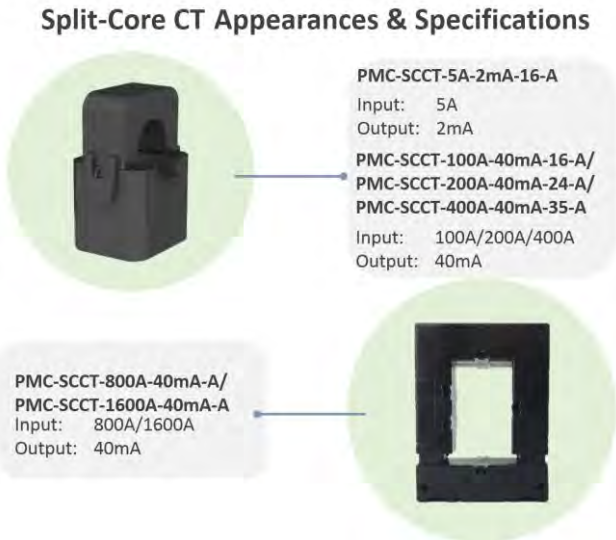
Figure 2-2 Split-Core CT Appearances & Specifications
