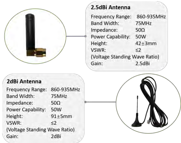
Figure 2-3 Antenna Appearances & Specifications
