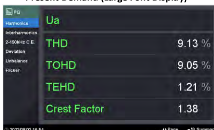
Voltage Harmonics (Large Font Display)
