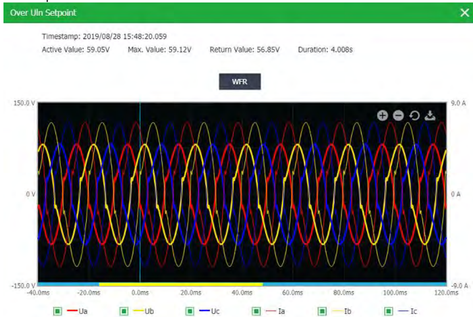
Figure 3-107 Over UII Setpoint
