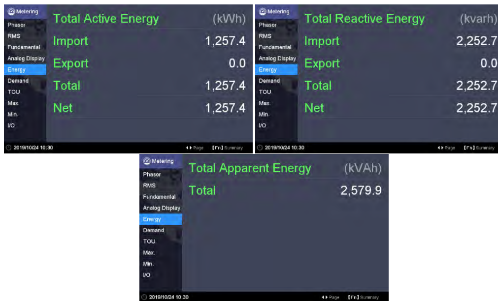
Figure 3-11 Large Font Displays for RMS Energy Measurements
