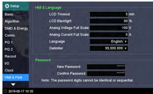
Figure 3-50 HMI & Pwd Setup
