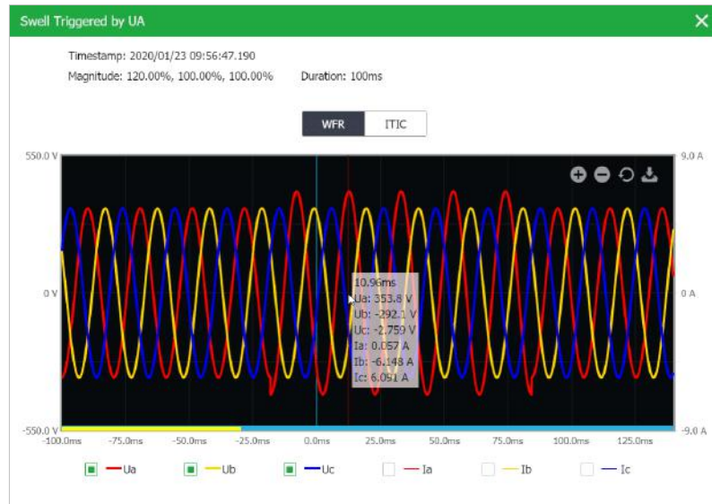
Figure 4-9 Swell Event @ 1024 samples/cycle x 40 cycles
