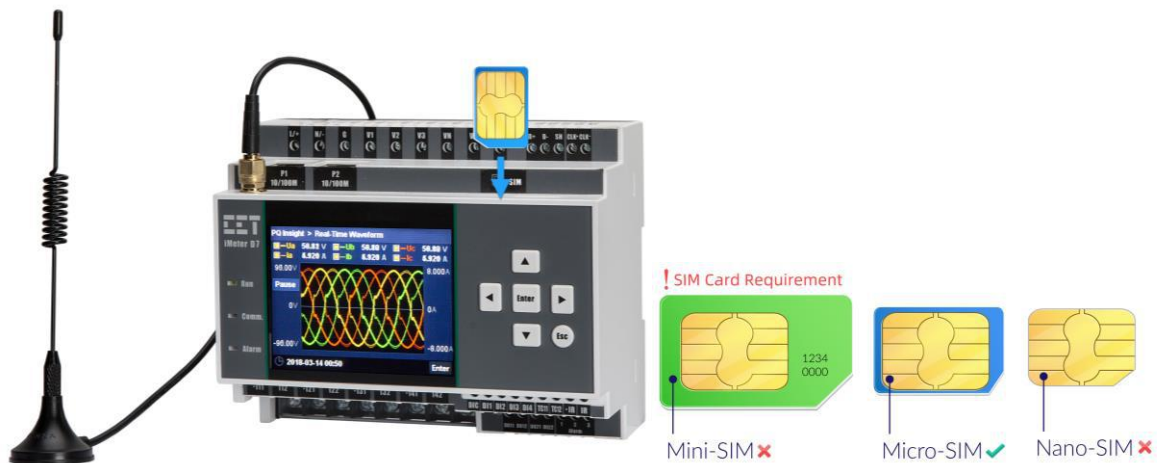
Figure 2-12 SIM Card Installation
