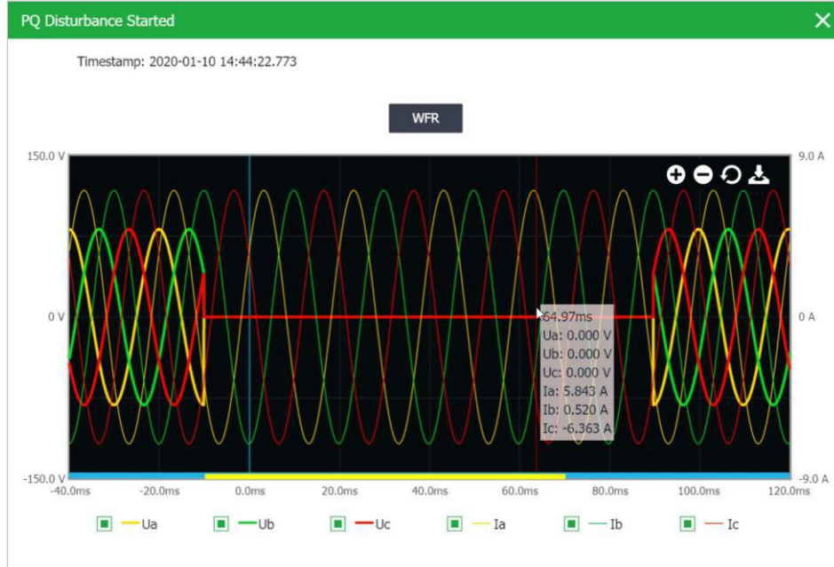
Figure 3-99 PQ Disturbance Started (Interruption triggered by UA)
