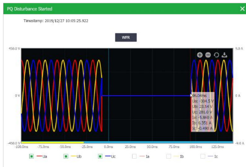
Figure 4-10 Interruption Event @ 1024 samples/cycle x 40 cycles
