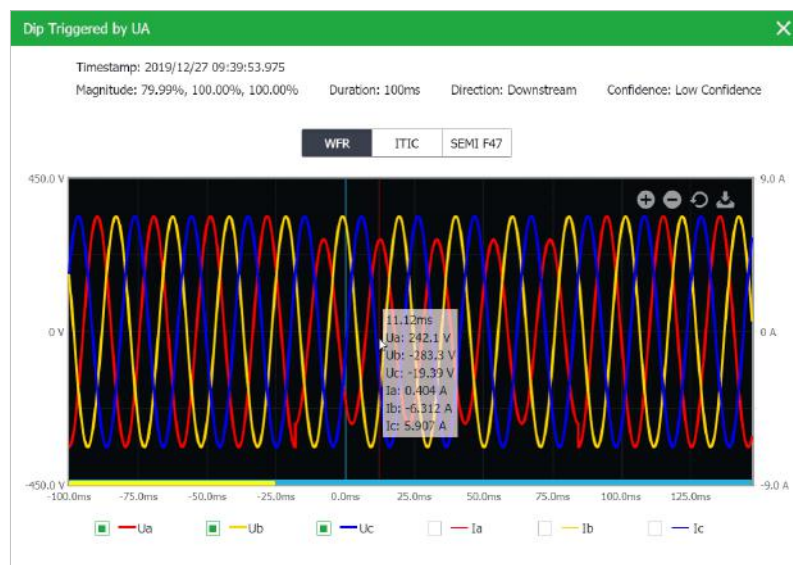
Figure 4-8 Dip Event @ 1024 samples/cycle x 40 cycles
