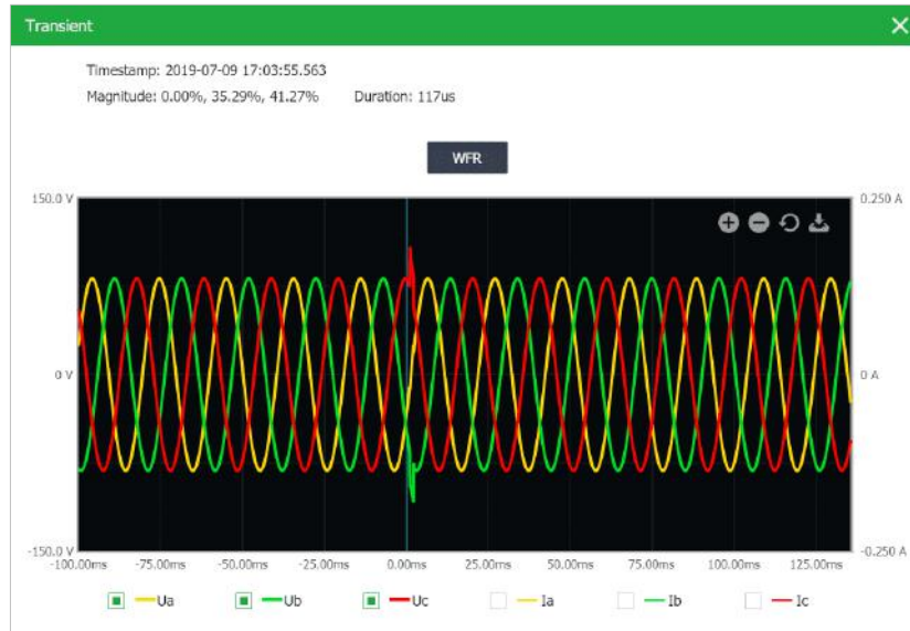
Figure 4-11 Transient Event @ 1024 samples/cycle
